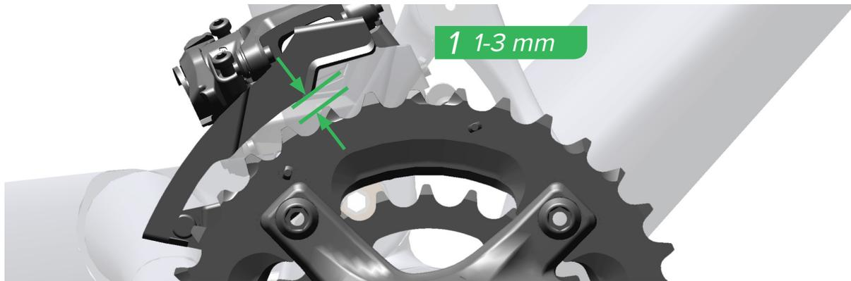
The distance between the top edge of the teeth on the large chain ring and the bottom edge of the derailleur cage must measure between 1-3 mm.
