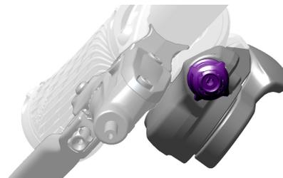
Slow shifting from a smaller cog to a larger cog (**inboard shifting**)? Turn the barrel adjuster counter-clockwise.
