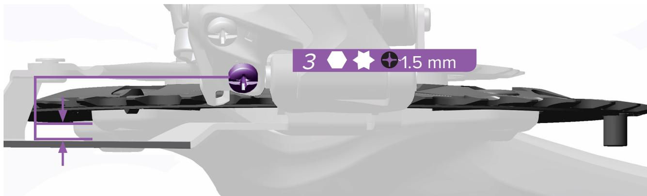
The distance between the outer edge of the largest chain ring and the inner edge of the derailleur cage should measure approximately 1.5 mm.
