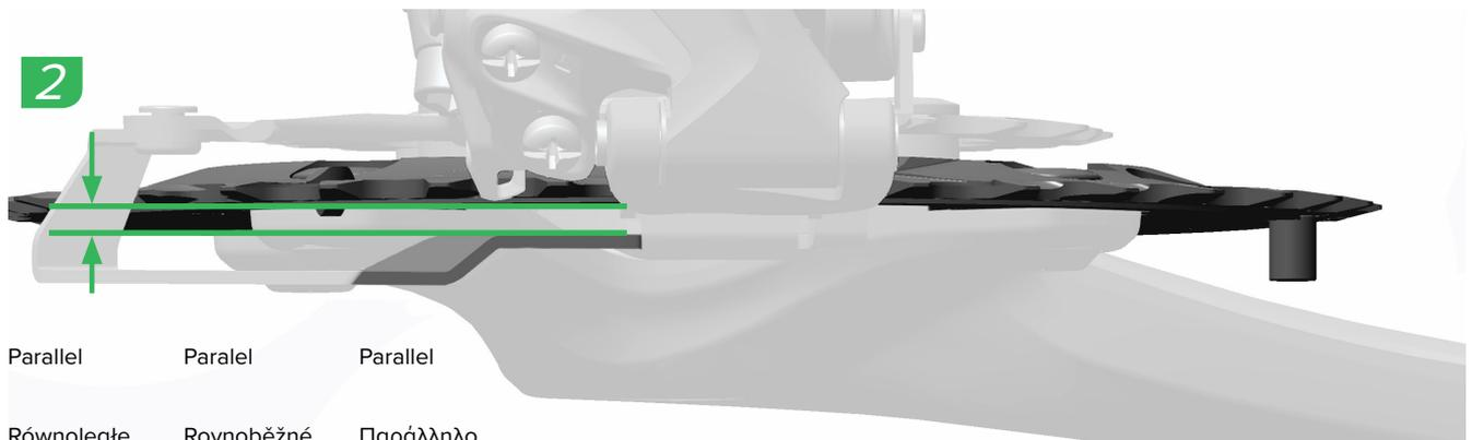
The largest chainring must be parallel with the inner edge of the outer cage.
