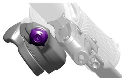
Slow shifting from a larger chainring to a smaller chainring (**inboard shifting**)? Turn the barrel adjuster clockwise.
