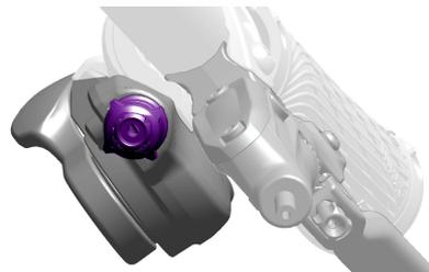
Slow shifting from a smaller chainring to a larger chainring (**outboard shifting**)? Turn barrel adjuster counter-clockwise.
