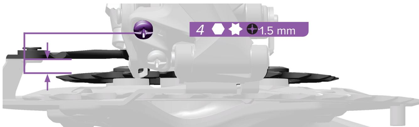
The distance between the outer edge of the smallest chain ring and the inner edge of the derailleur cage should measure approximately 1.5 mm.
